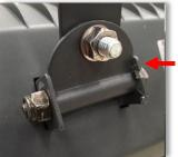
Heater bracket installed outside upper tab
