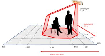
Radiant output has a strong centre that tapers off at the edges. There is no heat directly below the heater.
