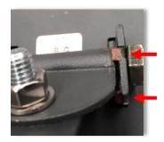
Heater bracket installed between upper and lower tabs.
