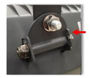
Heater bracket installed outside upper tab.
